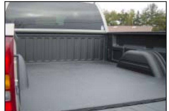
Combo Liners from pour-on and spray-on techniques, produce a heavy-duty bedliner with a flat floor
